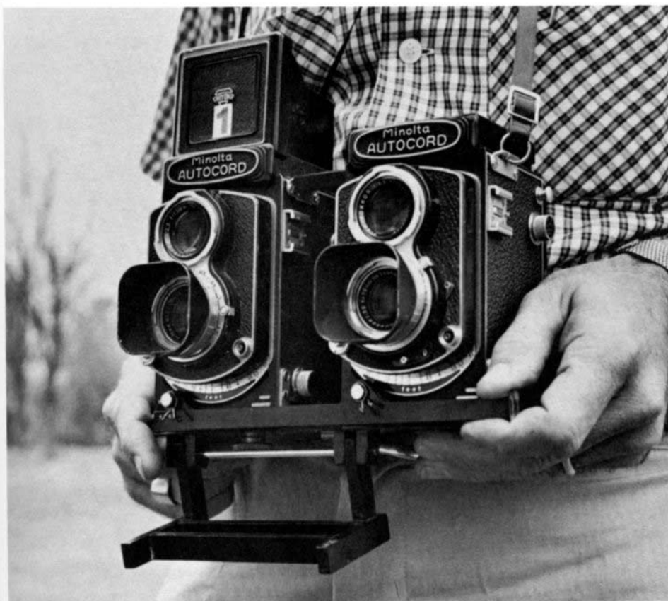
Two twin-lens Minolta cameras linked for simultaneous shooting with two different film types, or at two different shutter speeds, for special effects. The focusing levers are connected so adjusting one camera assures sharp focus for both; the bracket on the bottom swings up to set off both shutters nearly simultaneously.
